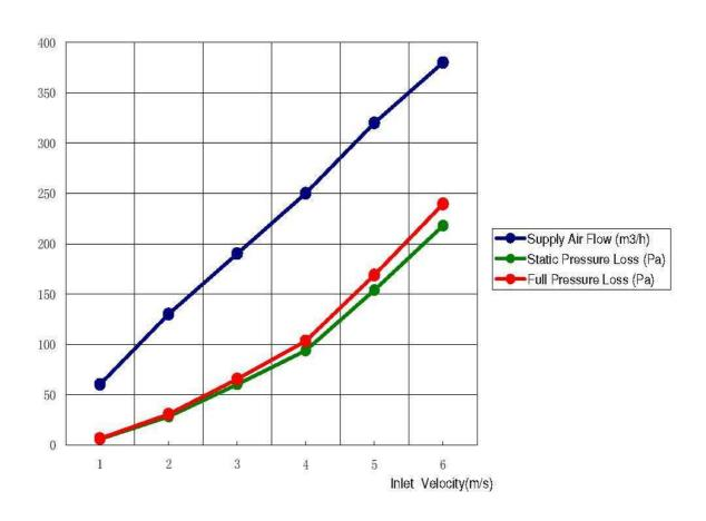
Remarks: 1.Above Table, Pressure Loss Included Resistance caused by 8 Leafs and Wire Net 2.Tested by National Center of Quality Supervision and Inspection and Testing for Air Condition Equipment.
